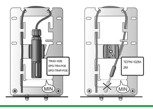
If the probe cable is too thin (approx. 2 to 3 mm, eg for the AT-TG3 probe) and there is a risk of instability of the probe sensor, secure the probe cable by turning the probe holder. See pictures below.
